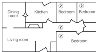
Figure 2: A SMOKE ALARM SHOULD BE LOCATED BETWEEN THE SLEEPING AREA AND THE REST OF THE DWELLING UNIT AS WELL AS IN EACH BEDROOM.
