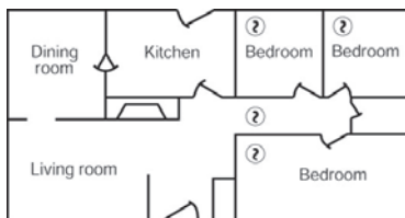
Figure 2: A SMOKE ALARM MUST BE LOCATED BETWEEN THE SLEEPING AREA AND THE REST OF THE DWELLING UNIT AS WELL AS IN EACH BEDROOM.
