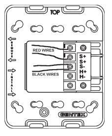
**CAUTION:** A jumper card is provided to test for correct wiring in the supervisory mode only. DO NOT pass alarm current through the jumper.
