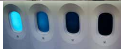
Above: Window control switches in production Right: Airplane window dimming stages
