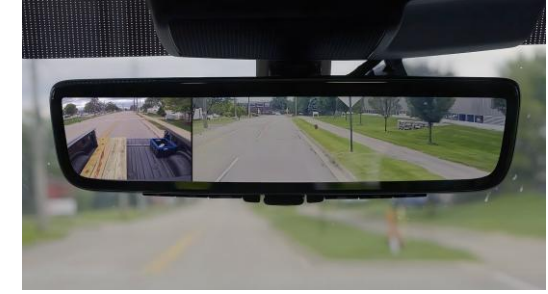
BED CAM VIEW (shows pickup bed and rearward view)
