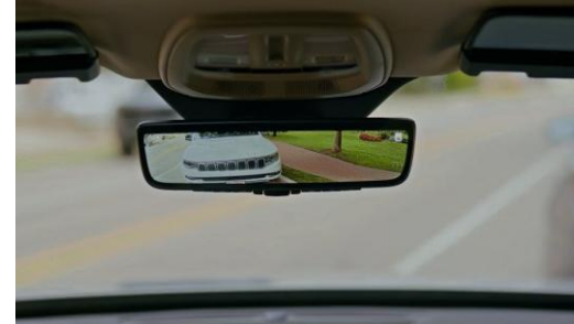
REVERSE ASSIST (pans downward while reversing)
