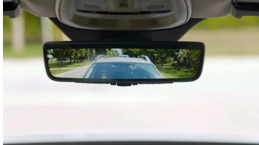
SPEED-ADJUSTED FIELD-OF-VIEW (adjusts FOV according to speed)
