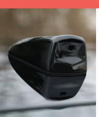
he Gentex Full Display Mirror (FDM<sup>®</sup>), is an intelligent rear-vision system that uses a custom camera and mirror-integrated video display to optimize a vehicle's rearward view. The system captures video from a rearward-facing camera and streams it to a unique mirror-integrated LCD that provides the driver with an unobstructed, panoramic view behind the vehicle.
