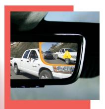
When in display mode, the driver can choose between various viewing modes that present the three camera feeds independently or stitched together to form a single, wide-angle view. The Gentex CMS solution can also work in conjunction with a vehicle's side blind zone warning system. When a trailing vehicle enters a side blind zone, a warning indicator illuminates in both the interior and exterior mirrors while the corresponding side-view video feed appears in the display until the vehicle passes.
